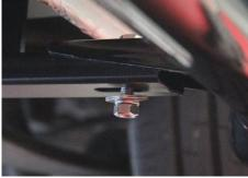
Important! After positioning the step in the appropriate position, tighten the M8 nuts with 25 Nm and the M10 nuts with 50 Nm.
