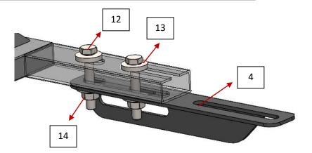
Important! After positioning the step in the appropriate position, tighten the M8 nuts with 25 Nm and the M10 nuts with 50 Nm.
