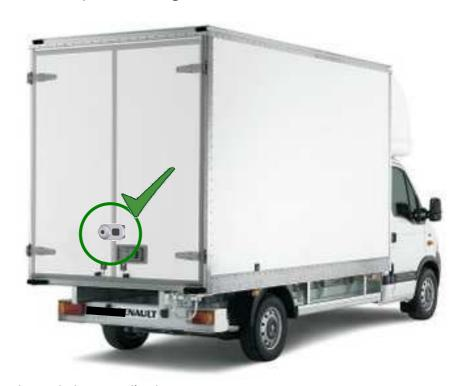
1. Apply the drilling template supplied.
