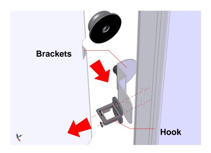
The type of fixation indicated previously, allows the application of the reversible lock. It will be possible to remove the plaque dedicated and tailgate will present the same characteristics as the original, avoiding costly steps to restore the vehicle body.
