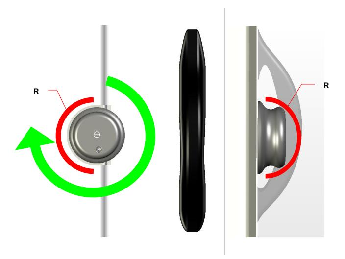
Thanks to its functioning (centering coupling on peg) the lock, once closed, can rotate freely on its axis preventing graspable actions to pull it off.
