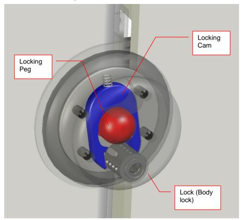
First, when the lock closes, the coupling between lock-peg makes a single body able to resist more effectively different attacks from burglary tools (hammer, chisel, crowar, pliers, screwdrivers..). In particular, the peg disappears inside the body lock making both a single part.
